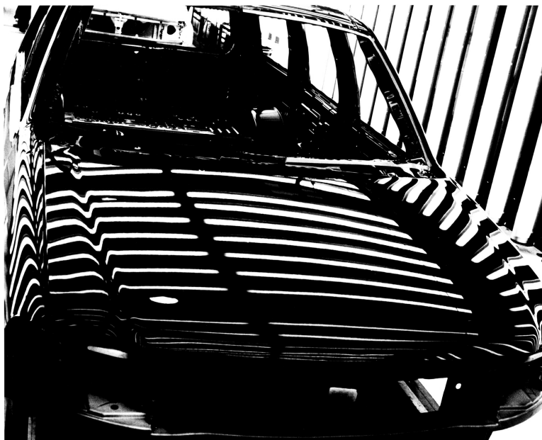
FIGURE 8.13 A lighting installation designed to make dirt defects in painted automobile body shells easier to detect. (Courtesy of Acuity Brand Lighting Inc., Atlanta, GA.)
