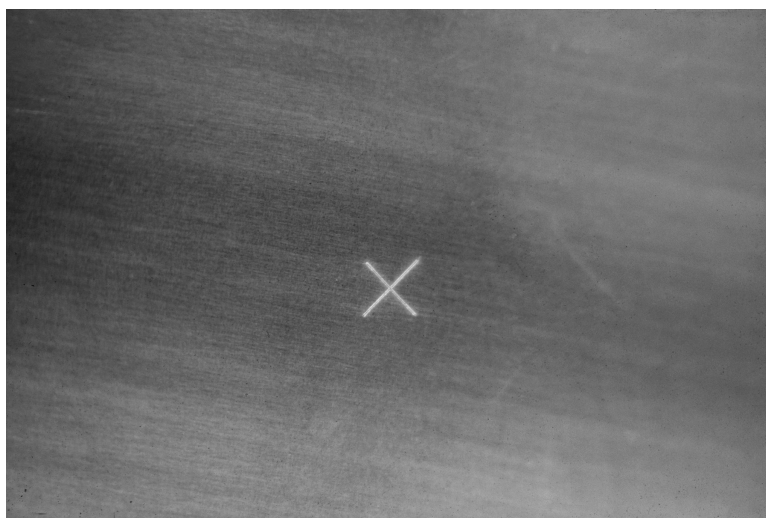
FIGURE 8.9 A specular aluminium surface with a cross scribed into it, lit by directional lighting from above and behind the camera. The scribed cross is easily seen because the scribed marks cut into the surface and thereby alter the reflection characteristics of the surface. The result is a high-luminance reflection towards the camera for the cut and a high-luminance reflection away from the camera for the undamaged surface.
