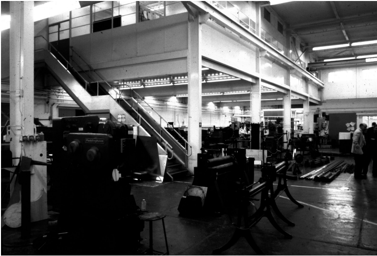
FIGURE 8.2 A small workshop with high-reflectance walls and lit by a regular array of luminaires with a wide luminous intensity distribution. The result is a shadow-free environment.
