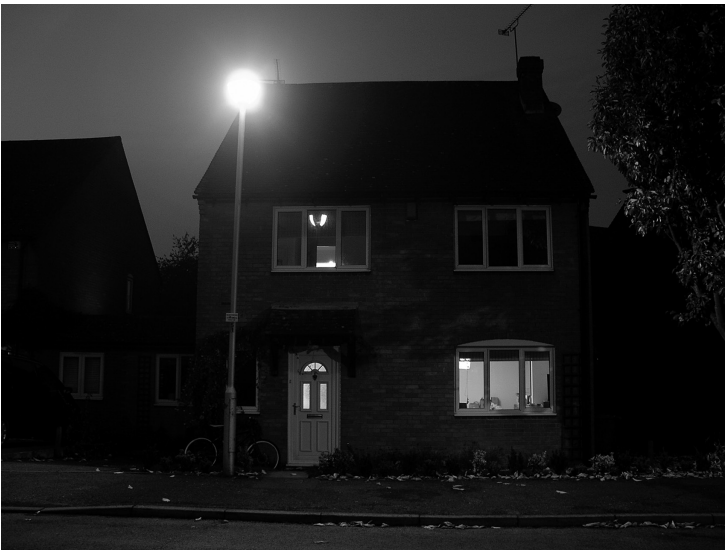
FIGURE 15.2 A classic light trespass situation. In this case, light trespass has been diminished by fitting the nearest luminaire with an internal house side shield. The house side shield can be seen in the image of the luminaire reflected in the bedroom window.
