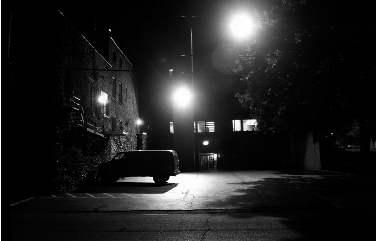
FIGURE 15.3 Disability and discomfort glare being produced by the building mounted floodlighting of an open car park.
